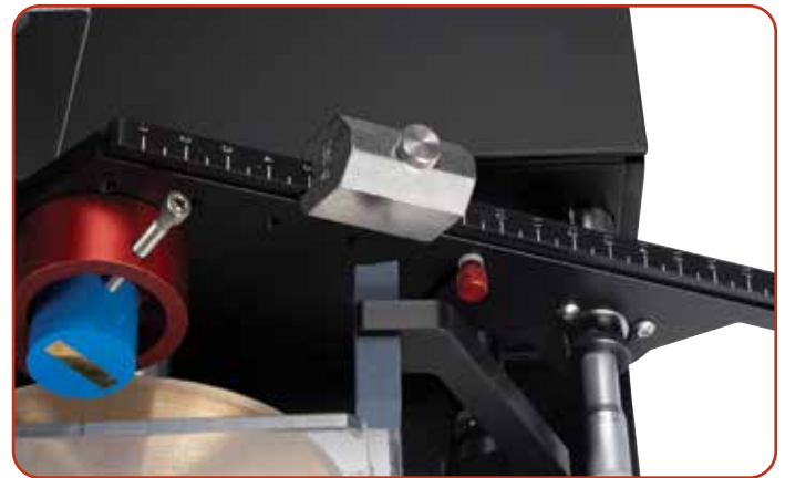
Sliding weights with graduated arm indicators provide variable load.
