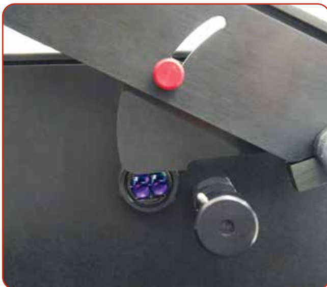
Optical shut-off sensor with adjustable stop
